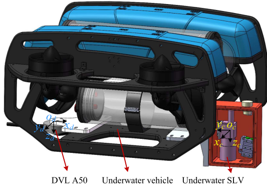
Fig. 1. Schematic diagram of experimental system.
